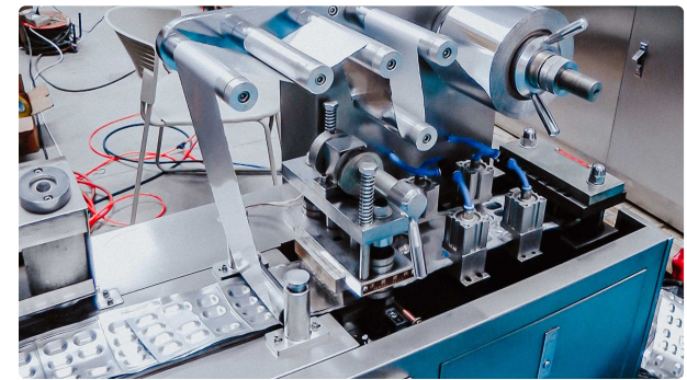
Automatic blistering machine for filling oval tablets into aluminum blisters
