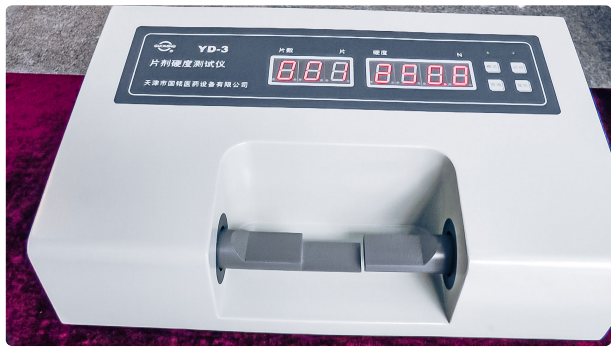
Automatic equipment for strength testing of tablets and pellets laboratory in pharmaceuticals...
