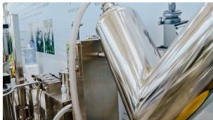
V Mixer for powder mixing and unloading to a vacuum conveyor
