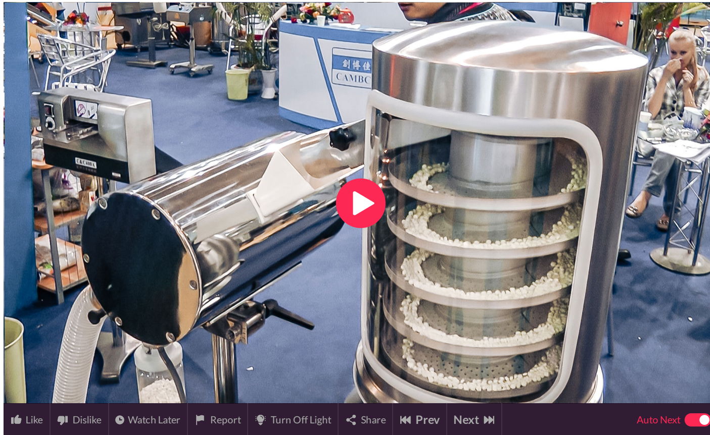
Automatic equipment for dedusting and polishing of tablets in pharmaceutical production
