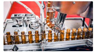
Automatic equipment for filling and capping penicillin bottles
