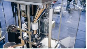
Automatic equipment for tablet pressing in pharmaceutical production
