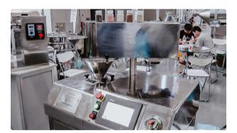
Granulator for pellet production pharmaceutical production of jelly and tablets
