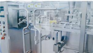
Automatic filling machine for dosing powders and granules into sachet bags
