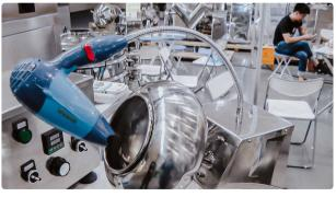
Laboratory machine for coating on jelly and tablet surfaces
