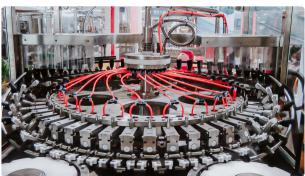
High speed automatic liquid drug bottling and capping machine
