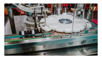
Equipment for high speed bottling and capping of liquids in spray nozzle bottles
