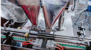
Automatic packing and capping of capsule and tablet in plastic bottles
