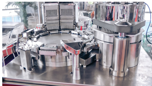
Automatic equipment for powder filling of gelatin capsules in pharmaceutical production
