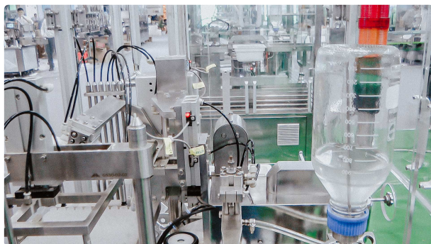
Automatic machine assembly and capping plastic syringes
