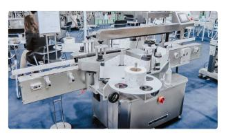
Automatic labeling equipment for sticking labels on glass bottles
