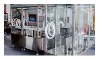
Monoblock bottling and capping laminar box penicillin bottles
