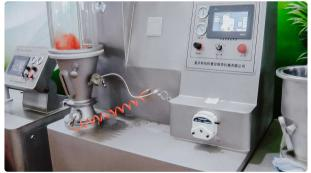
Laboratory equipment for drying and granulation in fluidized bed for pellet production
