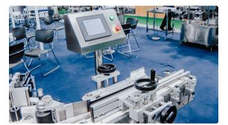
Pharmaceutical equipment for self-adhesive labels on penicillin bottles
