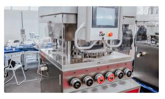
High speed automatic rotary tablet press for powder pressing
