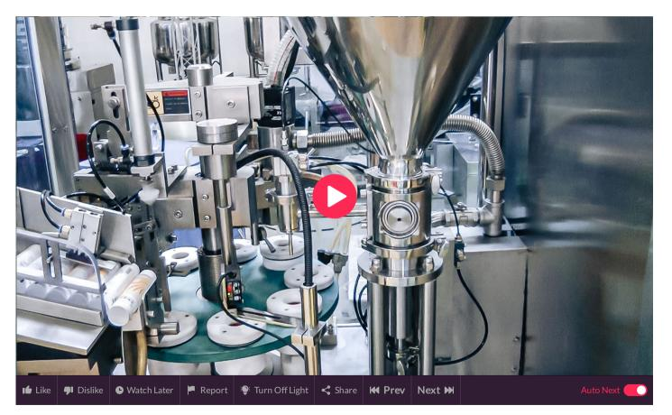
Automatic equipment for filling and sealing of cream in plastic tubes of pharmaceutical production
