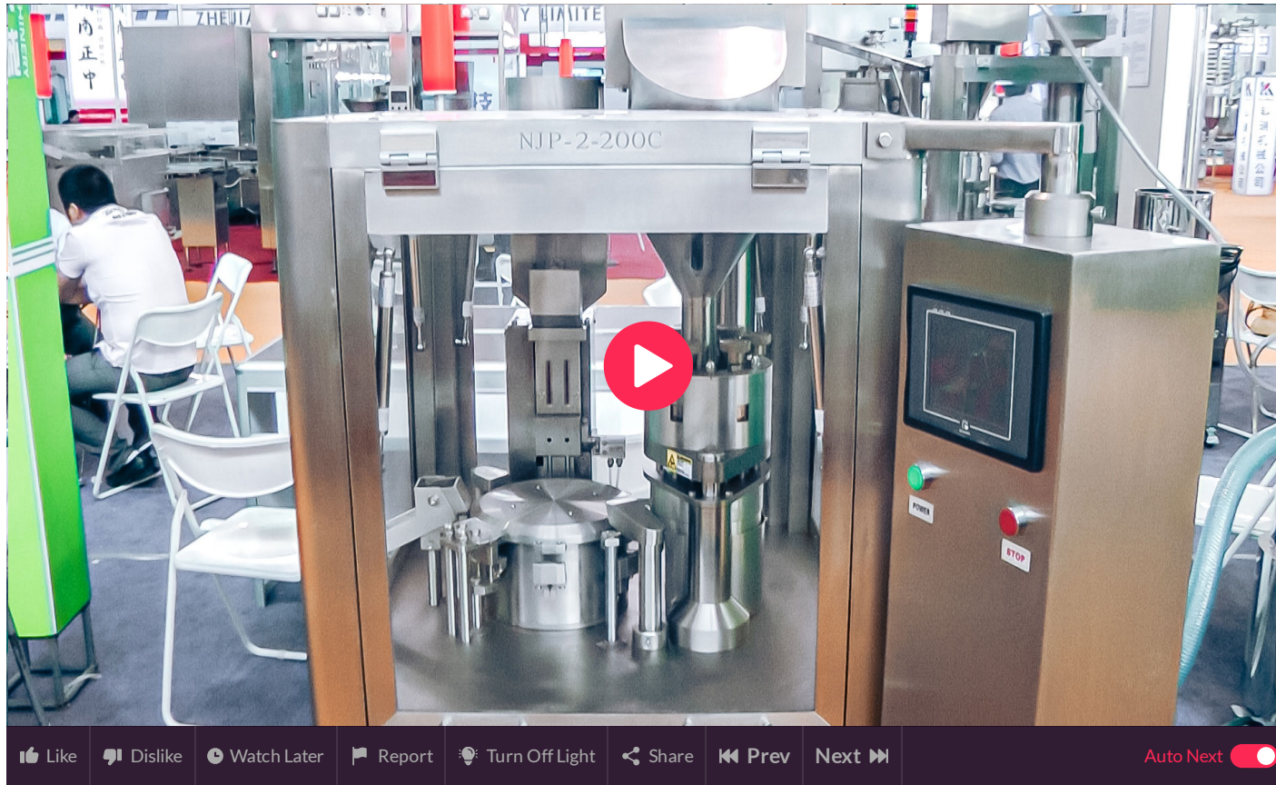
Automatic equipment for filling hard gelatin capsules with powder in pharmaceutical production
