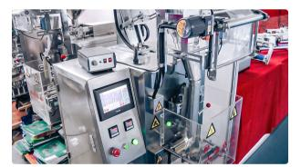
Automatic equipment for packing of products into sashet packs in pharmaceutical production
