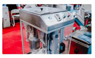
Automatic laboratory tablet press one punch for tablet production testing ITALY
