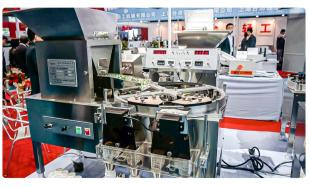
Automatic equipment for counting and packing of gelatin capsules into bottles Spain Pharmaceutical Tablet Press • 20.11.2020 • 78.477K views
