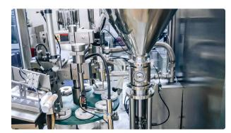
Automatic equipment for filling and sealing of cream in plastic tubes of pharmaceutical...
