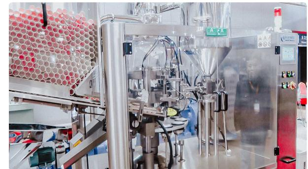
Automatic equipment for dosing and filling cream in plastic tubes with sealing
