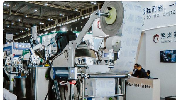
Automatic packing machine for packing powders and granules into pillow bags
