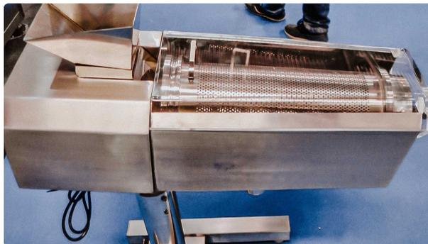
Automatic surface dust removal machine hard gelatin capsules vacuum cleaner
