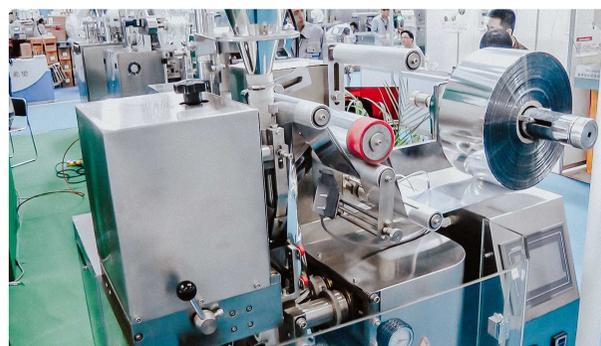
Automatic equipment for filling and packing powders in plastic bags
