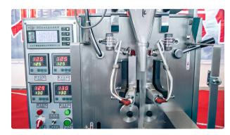
Automatic equipment for packing and packing powders into plastic bags in pharmaceutical...
