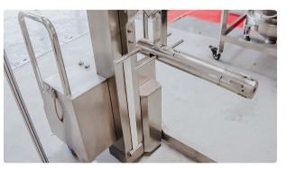
Automatic equipment for lifting containers with powders in a pharmaceutical factory
