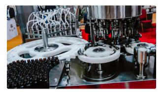
High speed automatic bottling and capping machine penicillin bottles
