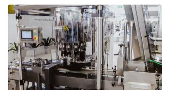
Automatic capping machine plastic caps with high speed for plastic bottles
