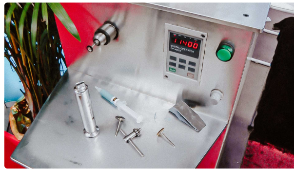
Polishing metal surface of the punch and matrix for pressing tablets
