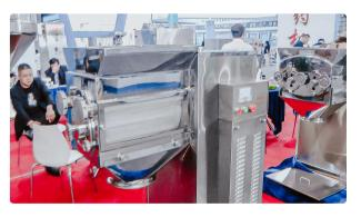
Granulator for the production of granules for tablet powders
