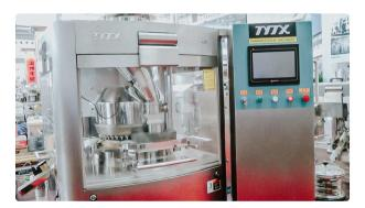
High speed automatic rotary tablet press for tablet production
