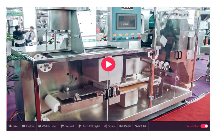
Automatic equipment for packaging of tablets and capsules in PVC blisters in pharmaceutical production
