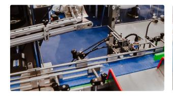
High speed automatic filling line of gelatin capsules in plastic bottles of silicogel pillows
