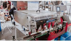
Automatic machine for filling hard gelatin capsules with powder into plastic bottles
