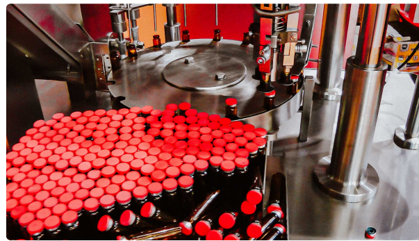
Automatic bottling and capping machine penicillin bottles with aluminum caps
