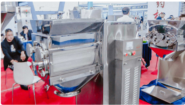
Granulator for the production of granules for tablet powders
