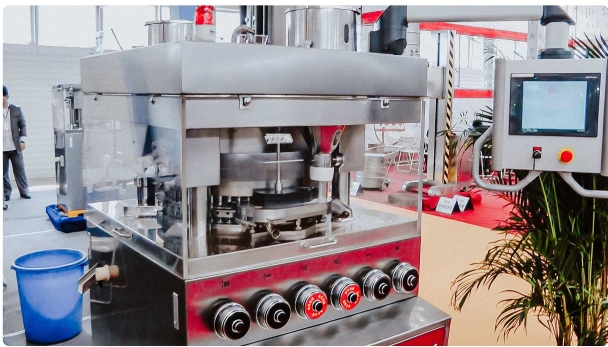
High speed rotary tablet press for pharmaceutical tablet pressing
