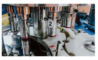
Automatic equipment for filling liquid products in a plastic syringe
