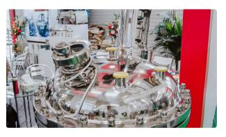
Stainless steel tank with water heating and mixer for preparing liquids and gel
