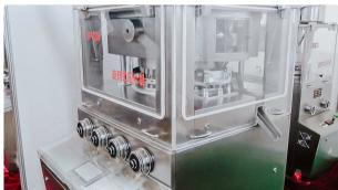
Automatic rotary tablet press for tablet production in pharmaceutical factory
