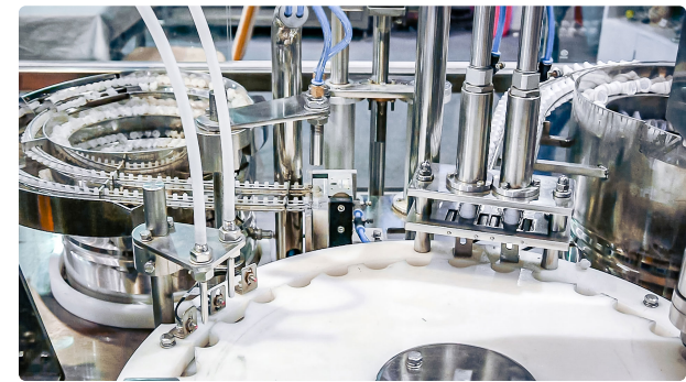
Automatic equipment for filling and closing of penicillin bottles aluminum caps
