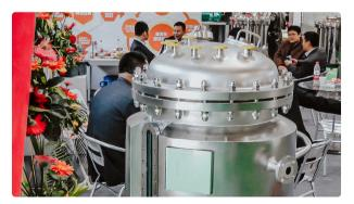
Tank for liquids volume of 200 liters with water jacket and heating for pharmaceutical liquids
