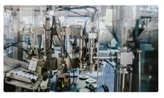
Aluminum and plastic tubes filling cream and ointment sealing
