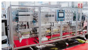
High speed automatic liquid filling machine in soft plastic ampoules
