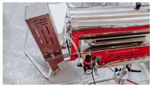
Automatic machine for polishing and dust removal from tablets and gelatin capsules with...
