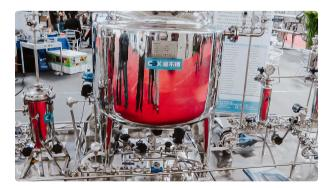
Cream and gel cooking homogenizer with heated mixer and water jacket USA
