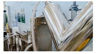
V Mixer for powder mixing and unloading to a vacuum conveyor
