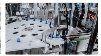
Plastic bottle filling and capping line with screw caps for liquids
