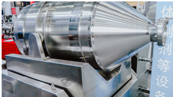
Powder mixer for food and pharmaceutical production
