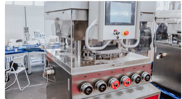
High speed automatic rotary tablet press for powder pressing
