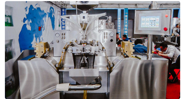
Encapsulation automatic machine to produce soft gel capsules for omega
