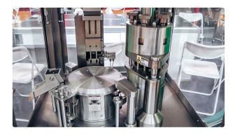
Automatic equipment for packing powder into gelatin capsules in pharmaceutical production Pharmaceutical Tablet Press • 09.12.2020 • 97.541K views
