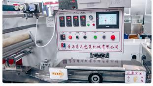
Automatic equipment for packing in cellophane in pharmaceutical production
