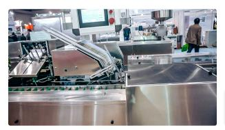
Automatic line for sticking self-adhesive labels on glass penicillin bottles
