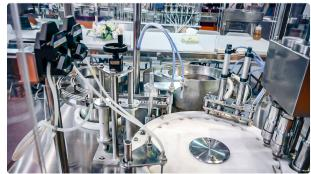
Automatic equipment for filling liquids into bottles in pharmaceutical production Pharmaceutical Tablet Press • 24.11.2020 • 177K views
