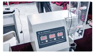
Automatic equipment for testing gelatin viscosity in pharmaceutical production USA Pharmaceutical Tablet Press • 08.12.2020 • 145.100K views
