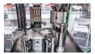
Automatic equipment for packing powder into gelatin capsules in pharmaceutical production
