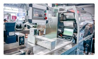
Automatic equipment for packing tablets and gelatin capsules in PVC blisters
