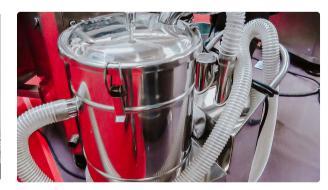
Automatic Powder and Pellet Dust Removal Machine, to work with tablet press
