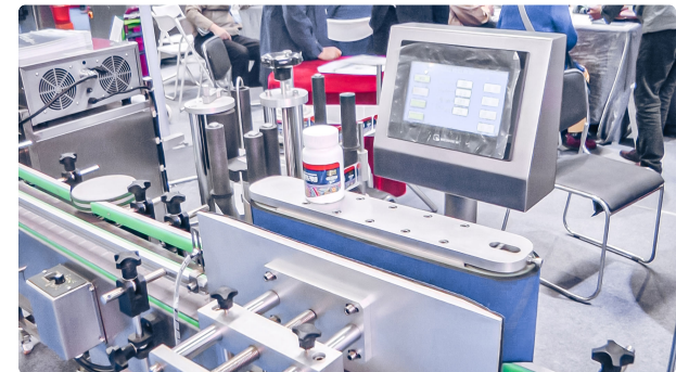
Automatic labeling equipment for plastic and glass bottles
