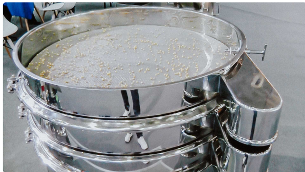
Vibrating sieve multiple levels for pharmaceutical powder fractions
