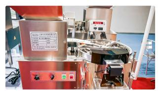
Automatic equipment for counting and packing of gelatin capsules into bottles
