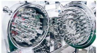
Automatic equipment for grinding raw materials and powders in pharmaceutical production...
