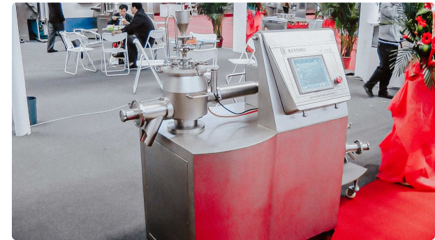
Granulator extruder for granulating powders in pharmaceutical production of medicines
