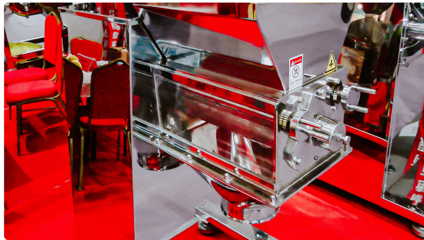
Granulator for the preparation of pellets in the cosmetic and pharmaceutical industry
