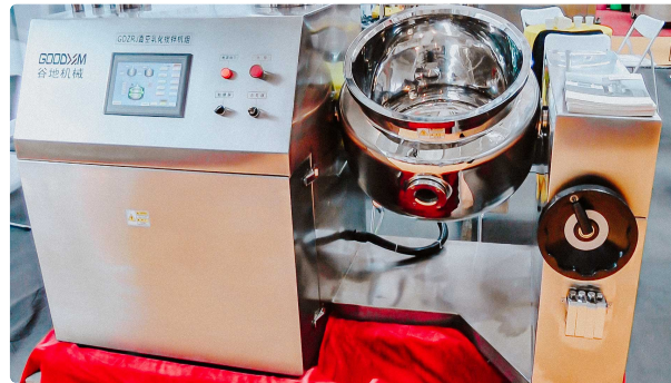
Pharmaceutical tank with heating and agitator for preparation of solutions and gels...
