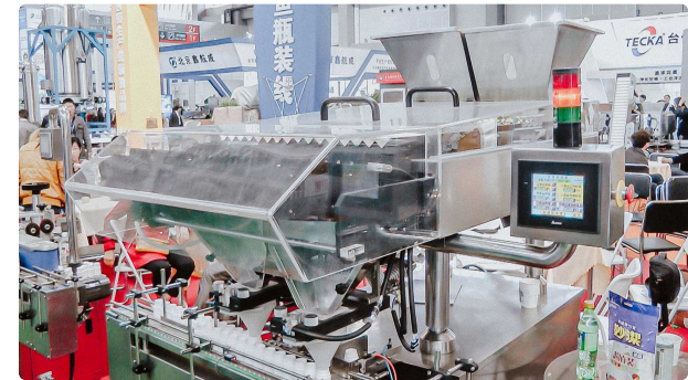
Counting and packing machine for packaging tablets and gelatin capsules in plastic bottles...
