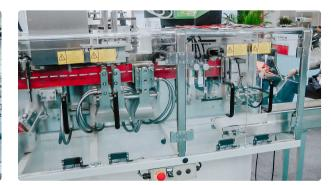
Automatic line for the production of wet wipes with alcohol individual package USA
