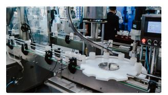
Equipment automatic powder dosage into plastic bottles and capping
