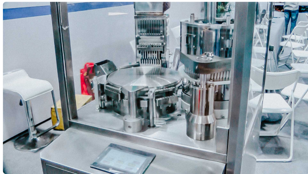
Hard gelatin capsules fill powder automatic drug making machine
