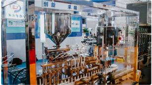
Automatic glass bottle filling and capping line machine for pharmaceutical production
